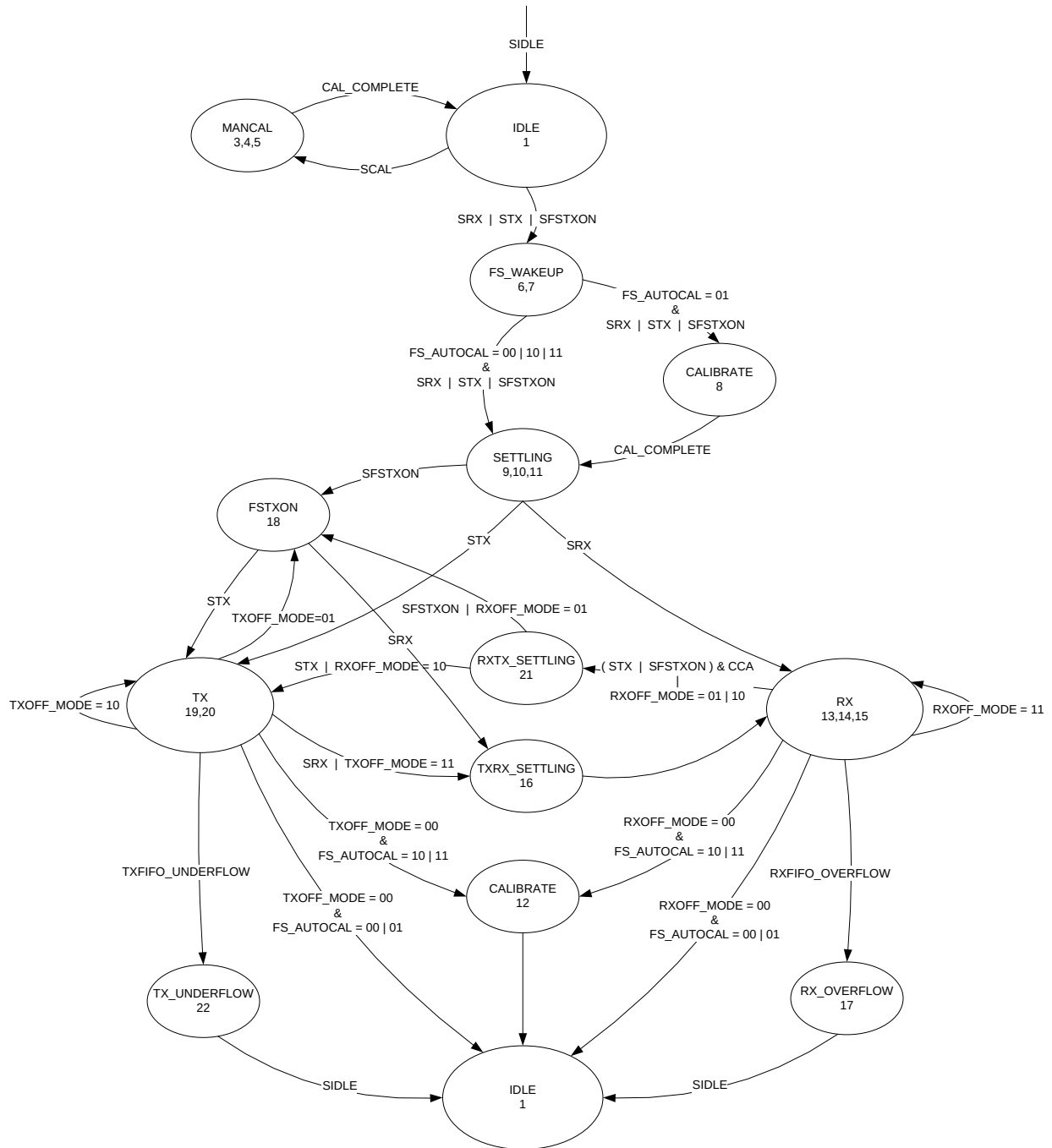
Figure 55: Complete Radio Control State Diagram
